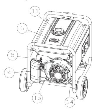
Figure 5 - Generator Controls
